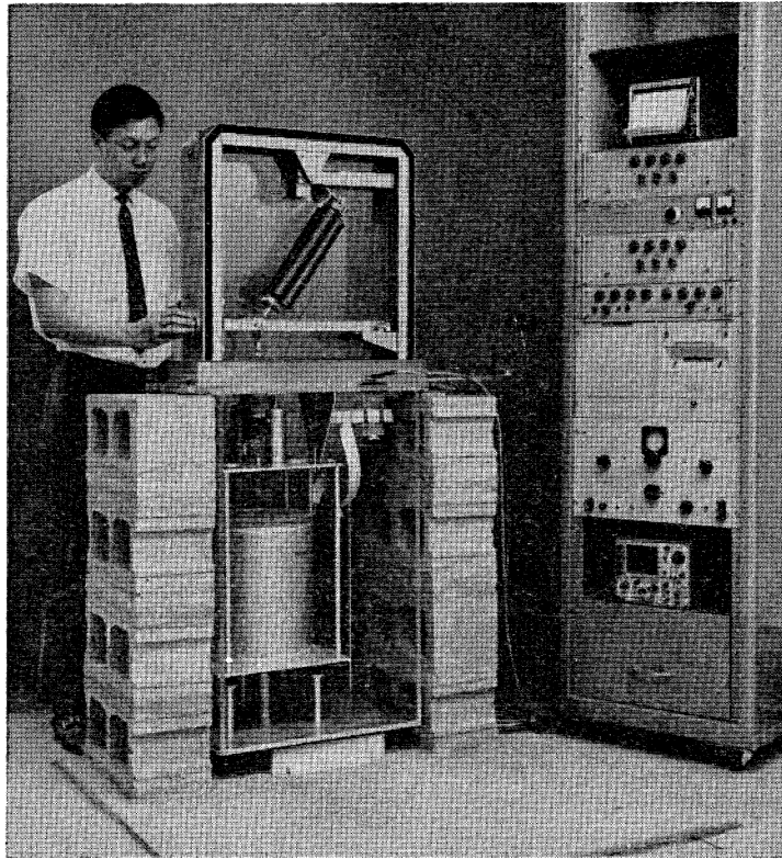
FIGURE 1. The final version of the calibrator being assembled for operation. A gravimeter (similar to TRG-1 gravimeters) is suspended from the beam of a modified long period seismometer.
